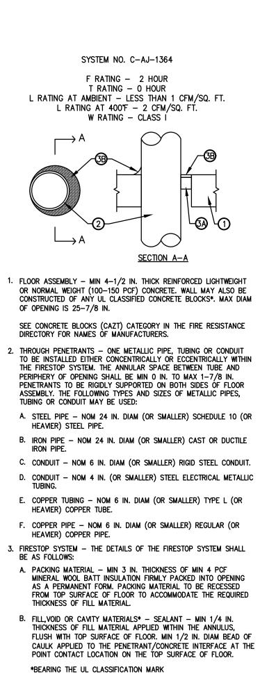
3M COMPANY - FB-1000 NS, FB-1003 SL OR FB-3000 WT SEALANT. \*BEARING THE UL CLASSIFICATION MARK
