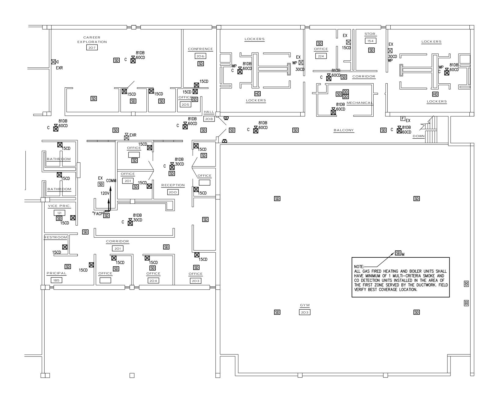
**PARTIAL FIRST FLOOR PLAN - FIRE ALARM** SCALE: 1"=10'-0"
